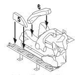
Figure 48 - Installing Logs No. 5 and No. 6
